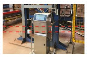
A UK based brick and concrete producer uses PrinterNet to remotely access their Linx 8900 printer located outside a safe area of their factory. The production line stops if the light beams in front of the printer are broken so being able to create and amend messages remotely is a perfect
